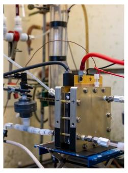
Our first step to reduce the cell resistance is to understand the composition of it. One of our skills is to diagnose the battery cell *in-situ* and identify the factor(s) limiting the battery performance using electrochemical impedance spectroscopy (EIS). Understanding the dominating factor(s), will facilitate how to improve the battery performance.
